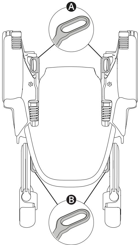
The wheelchair is equipped with four tie-down points used for transportation. Two in the front **A** and two in the rear **B**.
