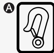
After you have secured the straps to your wheelchair, secure the other end of the straps to your vehicle according to the appropriate instructions. The end-fitting on the strap must comply with ISO 10542–1:2012, which is an international standard that governs wheelchair tie-downs and occupant-restraint systems. Every vehicle tie-down system is different, and it is important that you follow the instructions for your particular vehicle system.
