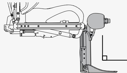
1. Make sure that the leg rest is in its most vertical position.
