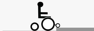
When you drive downhill, additional precautions must be taken. Select the lowest maximum speed and proceed with caution. Driving down a slope can shift your center of gravity forward. Release the joystick if the wheelchair rolls faster than you would like. This makes the wheelchair stop, and you can descend again more slowly. Avoid sudden stops and starts. Note that the distance required to stop will increase when you drive downhill.
