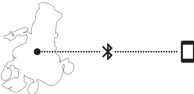
Your power wheelchair has a Power Platform, which contains a radio transmitter. In certain areas, radio transmission is not allowed and your wheelchair must be set to flight mode ✈.
